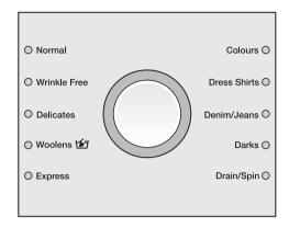
■ Turn the program selector right or left to select the desired program. A program is selected when the indicator light next to the program name is on.
